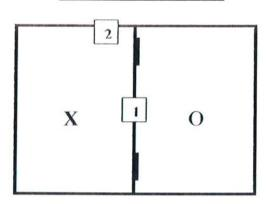
Deflection / Permanent Set were measured with two (2) Mitutoyo dial indicators SN- A066, and SN - A070
