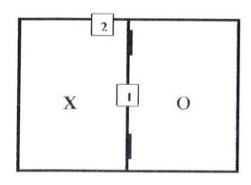
Location (1) - Max. Allowable Perm. Set after test load at center mid-span of the fixed meeting stile. (0.4% of 1556 mm (57.00°) span) = 6.2 mm (0.228°)
